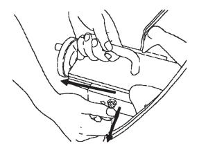
To remove the fetus support board, use your right hand to pull out the lock knob, grasp the handle with your left hand, and pull the board out towards you. Only the fetus support board will be pulled out.
