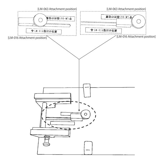
(2) Adjust the clamp arm to the appropriate attachment position, and then set the main body close to the clamp arm.
