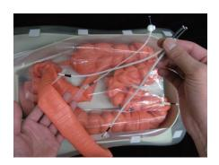
\* Insert the cords one by one, not both cords simultaneously, in the openings of the transparent cover of the main unit and the round stopper.
