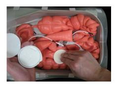
14) Pass the first cord from the ascending colon through the opening in the transparent cover of the main unit and affix it with a round stopper.
