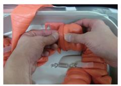
\* Make sure to align notch marks on each connector.
